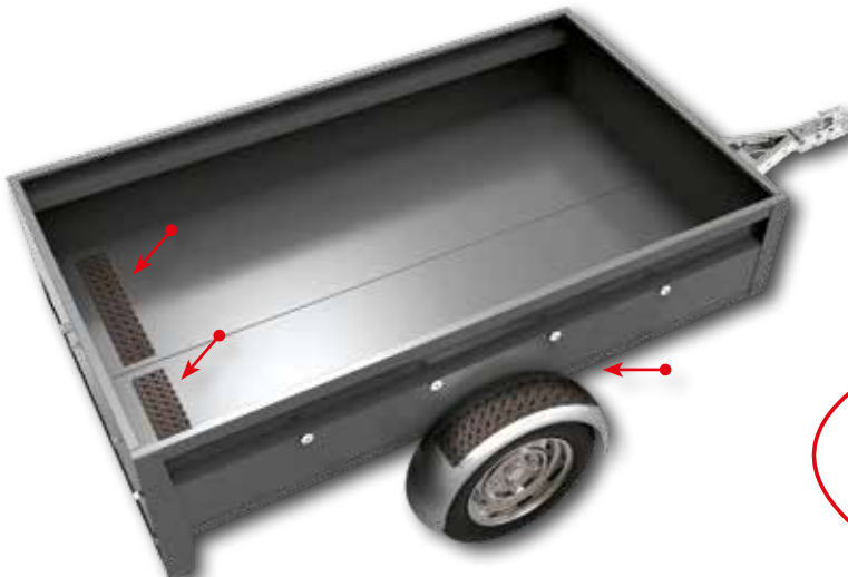
Self-adhesive step treads added for traction
