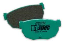
Friction Coefficient 0.50 - 0.55 Temperature Range 0 - 380°C
